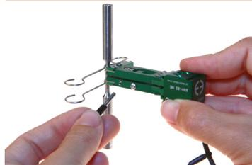
*Model 3442 low-profile extensometer with gauge length pin*
